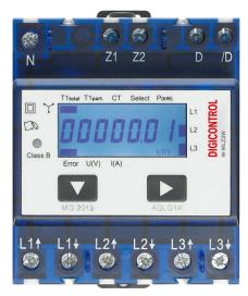
The electronic three-phase energy meters with M bus/Modbus RTU interface enable the reading of all relevant data like energy (total and partial), current, voltage and active and reactive power.
