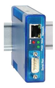
The DC-COM-Serv is used as carrier protocol converter for converting a standard M-Bus or Modbus to Ethernet TCP/IP. The serial interface of the server can be switched between the standards RS232, RS422 and RS485. 1x Com-Server Highspeed Industry and 1x product CD are included in the scope of delivery.
