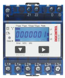
The electronic three-phase energy meters with M-Bus/Modbus RTU interface allow reading of all relevant data, such as energy (total and partial) current, voltage, active and reactive power.
